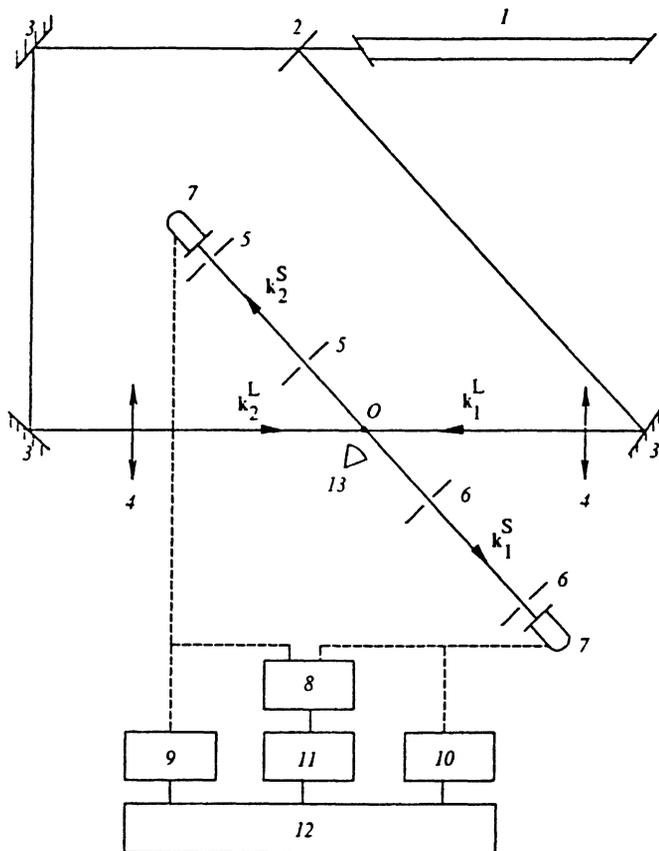
FIG. 2. Sketch of experimental setup for investigating intensity correlations for elastic light scattering.  $k_{1,2}^S, k_{1,2}^L$  are the modes of scattered radiation and pump. 1—Ar<sup>+</sup> laser; 2—beam splitter; 3—rotating mirror; 4—long-focus lenses; 5, 6—irises; 7—photomultiplier; 8—coincidence circuit; 9, 10, 11—pulse counters; 12—microcomputer; 13—photodiode.
